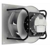
Motor is internally mounted integral to an isolated fan assembly. Standard motor shall be horizontal foot mounting, induction motor, squirrel cage, totally enclosed fan-cooled (TEFC or TEFV) with IP 55 protection and class F insulation. Motor capacity cannot be undersized but oversized for desired running capacity. For the desired operation speed between fan and motor, different poles (2, 4, 6 and 8 poles) can be consider.
